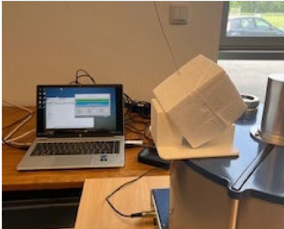
Photo 2. GRUAN humid room check along with the connected logiciel to record examined sounding data.
